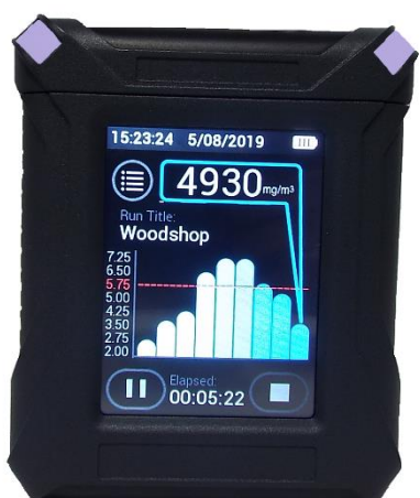
Figure 3-16. Flow Faults cause purple lights to flash
