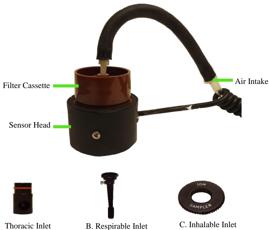
Figure 3-2. Diagram of sampling inlets for Thoracic, Respirable, and Inhalable. Pictures are not to scale.
