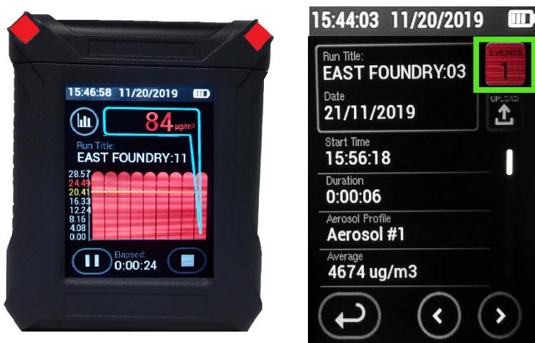
Figure 3-17. Battery Faults cause red lights to flash
