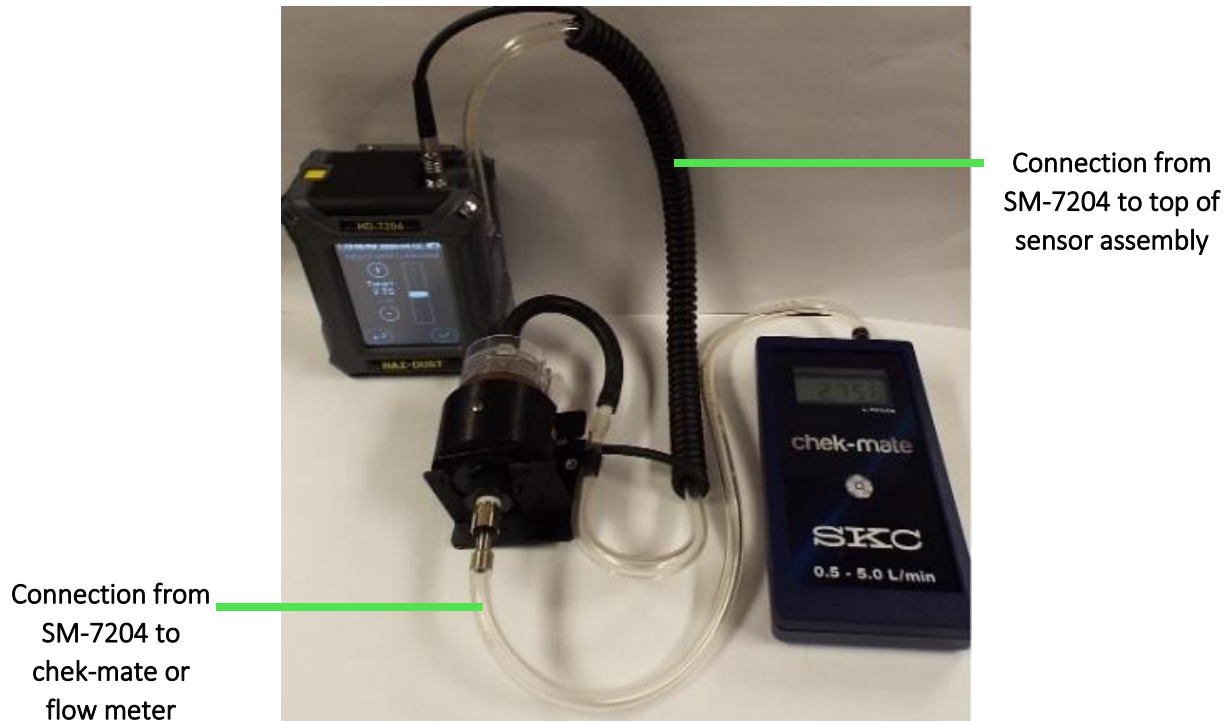
Figure 3-12. Connecting SM-7204 to SKC chek-mate
