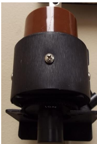
Figure 3-15. CS-7204 being inserted into SM-7204 sensor
