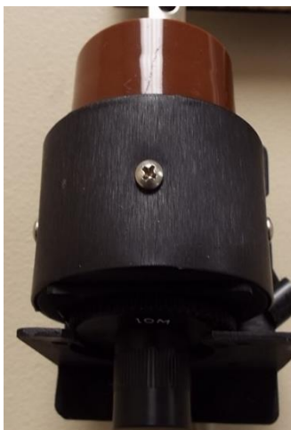
Figure 5-1. CS-7204 being inserted into SM-7204 sensor
